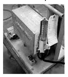
weld start in a survey made of a bar joist fabrication shop where needle valve control flowmeters were placed at the gas inlets on 100 MIG wire feeders to eliminate starting gas surge. The flowmeter had a scale calibrated at 50 psi inlet, which was the pressure in their bulk shielding gas pipeline.
